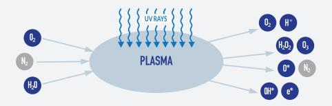
KVir-P uses innovative high intensity dual wavelength UV lamps that generate plasma, i.e. a gaseous mixture charged with energy and containing O+, O-, O2, O, O3, ionised O2, metastable excited O2 and free electrons. Plasma has the following effects:
